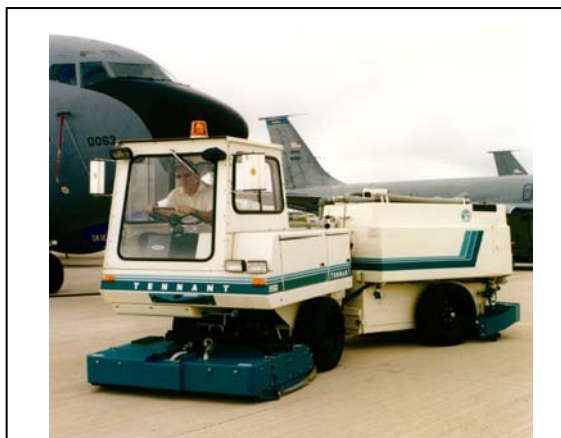
Deicing recovery vehicles remove deicing fluid from runways to prevent it from contaminating the base's creeks.
