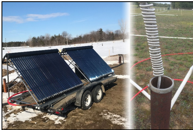
TISR Components: Solar Panel on Mobile Platform (L) and Borehole Heat Exchanger (R).
