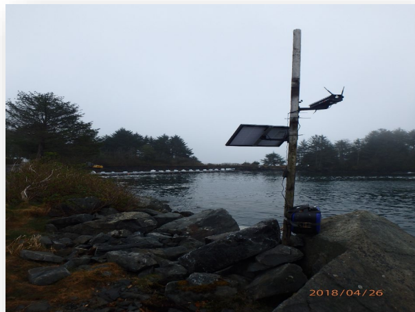
Photo 7: Internet-connected wireless remote camera used to monitor work progress, weather, and tides. This camera was available to the contractor and government 24 hours-a-day, 7 days-a-week. (2018, A. Shewman)
