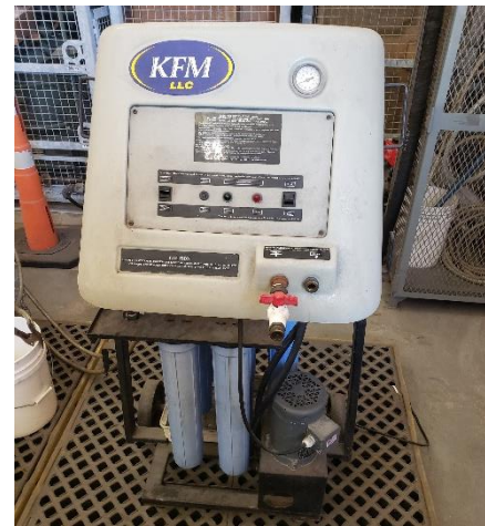
KFM, LLC coolant purification system used to recycle used antifreeze at MCSF-BI. Used antifreeze is collected by shop personnel and transferred into a used antifreeze tank at Building 350. Once a sufficient volume of has been collected, it is processed through the CPS and transferred into a purified antifreeze tank for dispensing to shops.
