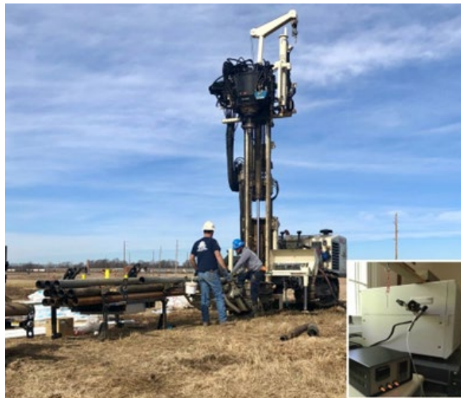
Figure 6. An expedited and dynamic characterization of Area 5 and Area 17D using whole-core soil sampling (WCSS) with an onsite direct sampling ion trap mass spectrometry (DSITMS) laboratory allowed LCAAP to identify an unknown groundwater source and establish detailed contamination assessment for targeted remediation that will optimize restoration timeframes.
