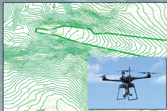
IR 7 ravine topography captured via LiDAR-equipped drone (inset)
