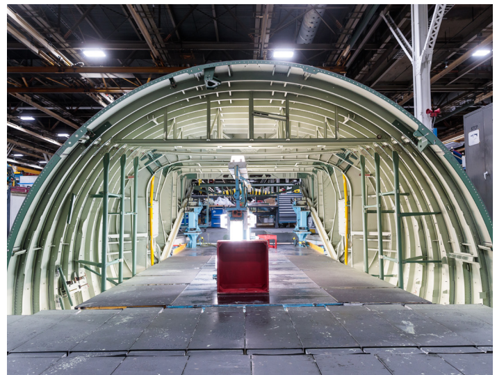
Interior view of a production C-130J with new non-hex chrome finish.
