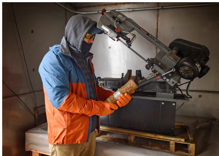
Ordnance and Explosive Safety Specialist Mr. James Ennis prepares a 75 mm munitions debris item for cutting on a remotely operated bandsaw, February 2021. Cutting a munition item is part of the process to render a munition safe.
