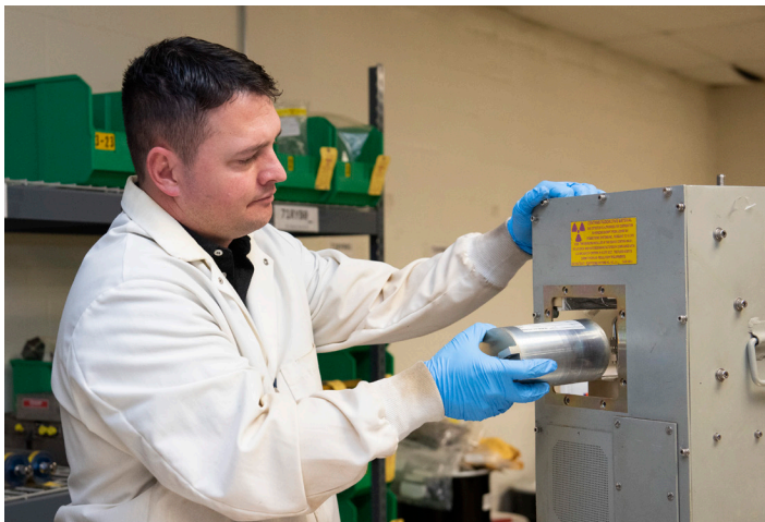
Mr. Seth Walton disassembles a Navy Shipboard Chemical Agent Detector Alarm.
