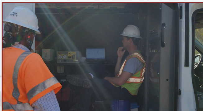
Real time MIHPT results allow for dynamic field events where locations can be selected and plumes delineated in minimal mobilizations without waiting on lab results.
