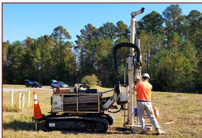
A MIHPT is advanced via a DPT generating little to no waste.
