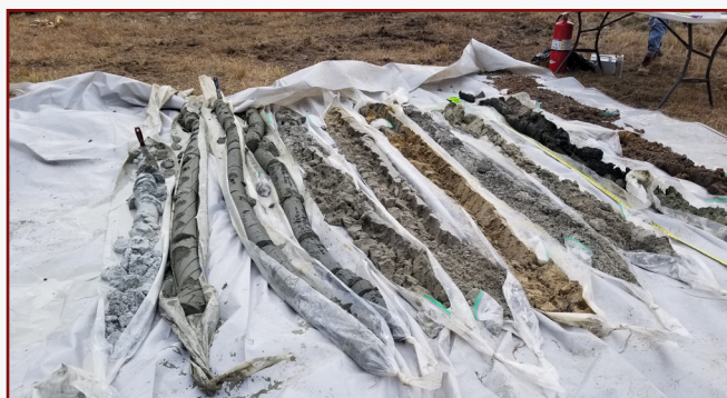
Confirmation soil borings were analyzed for VOCs, lithology, and soil geophysical/geochemical parameters.
