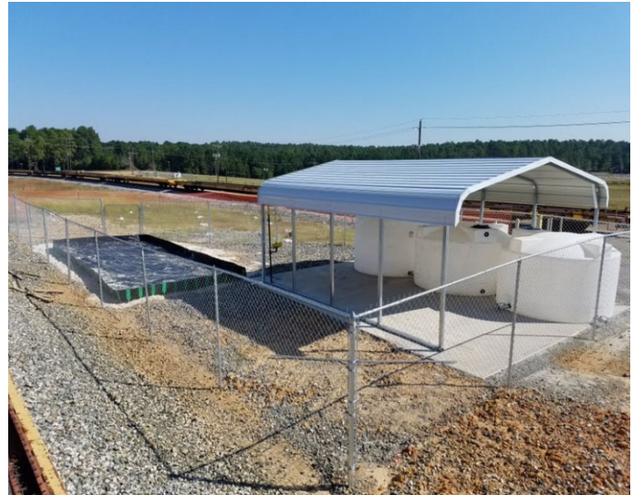
SWMU 26 Site showing the In-Situ Chemical Oxidation setup with temporary wells flagged in upper left prior to closure proceedings.
