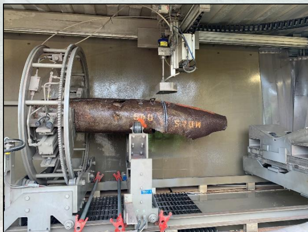
Figure 11. Water jet cutting system dismantling an inert practice bomb recovered during the munitions cleanup in Vieques. Processing inert munitions in this manner is a cost-effective way to enable the metal casings to be recycled for beneficial reuse.
