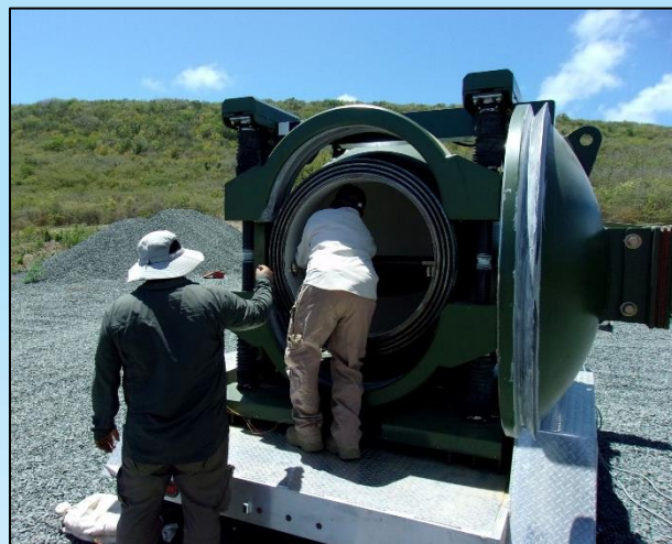
Figure 10. Closed detonation chamber being prepared for destruction of 20-millimeter projectiles recovered during cleanup of the former Vieques Navy training ranges.
