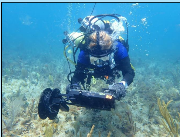
Figure 6. Teams of divers utilizing underwater navigation equipment search for munitions on and beneath the seafloor adjacent to planned public beaches as part of a novel characterization approach.
