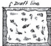
For both hard and soft stones. Rock or Pitch Face.
