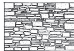
Laid of stratified stone fitted on job It is between rubble & ashlar. Finish is quarry face, seam face or split Called rubble ashlar in granite. SQUARED-STONE MASONRY
