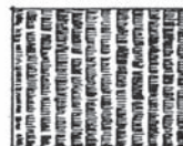
For soft stones. Tooth-chisel.
