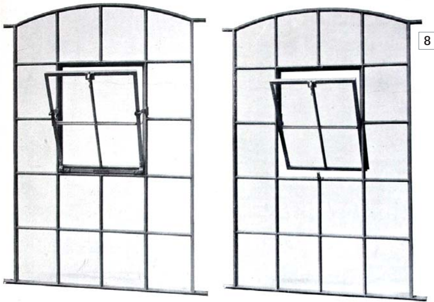
Henry Hope & Sons 1904 wrought steel windows were the predecessor to the more common rolled steel windows. The steel's strength allowed the character-defining feature of narrow muntins.
