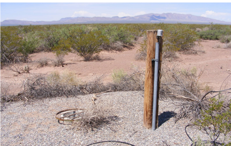
One extant grate with microphone and hole assembly (bottom left) at a SOTIM station on WSMR. (Photo by author)
