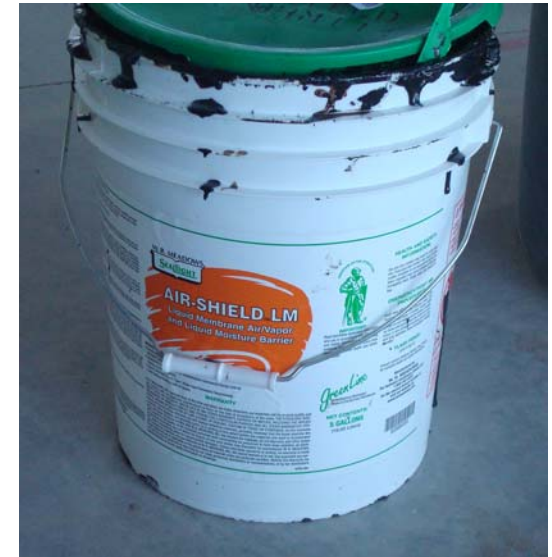
Figure 04 21-7 Liquid barrier, looks like black tar
