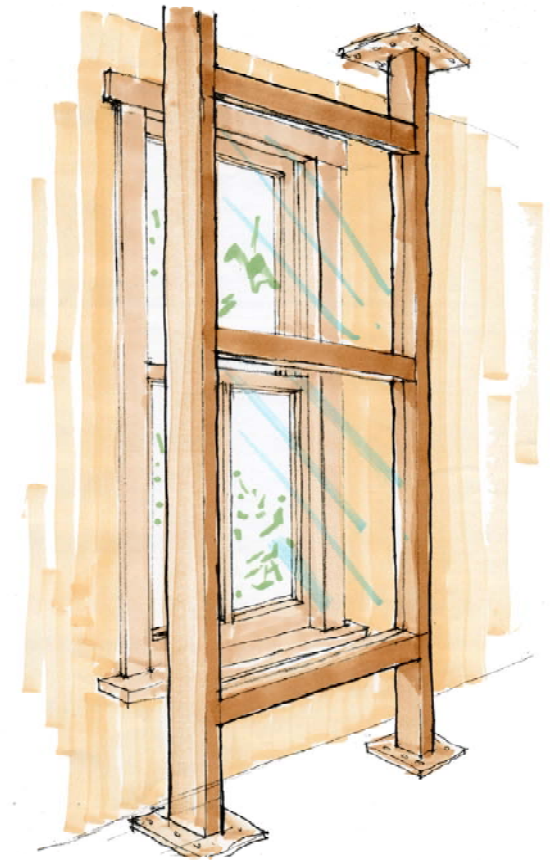
Figure 08 52-4 Possible solution for Force Protection and Anti-Terrorism at a historic building. Build a removable blast guard at the interior of the space, taking care to mimic the configuration of the existing windows.
