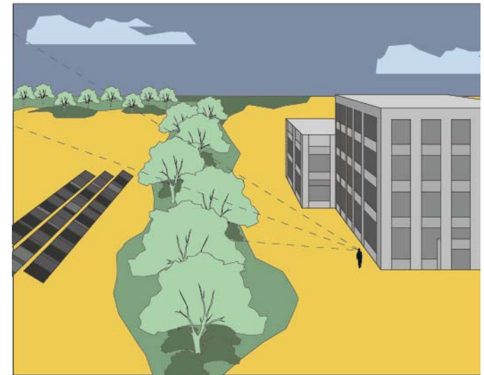
Figure 01 01-5 In a historic district, a good strategy to be used when adding a PV array would be to screen the PV array from the user with landscaping or fencing.
