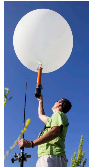
Rich Fischer deploys an Autonomous Aerial Acoustic Recording System (AAARS) at Fort Bragg, North Carolina. The AAARS is affixed to a weather balloon tethered from below and flown aloft, to compare avian point count data collected from a stationary ground-based observer with that of the AAARS. Source: Rich Fischer
