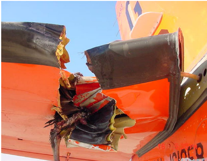
A T-45 aircraft involved in a crash with pectoral sandpipers at NAS Meridian, Mississippi. Source: U.S. Navy
