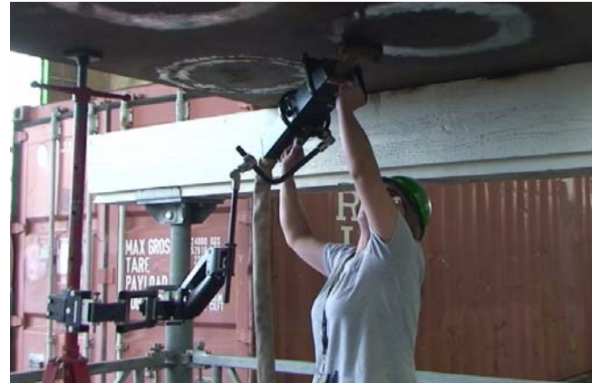
Equipos ZeroG TM * with induction heating unit I
