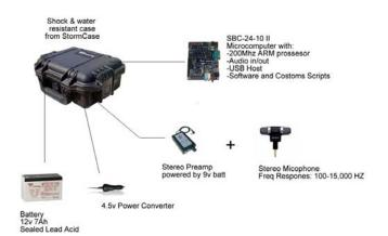
Figure 2. Portable recording station.
