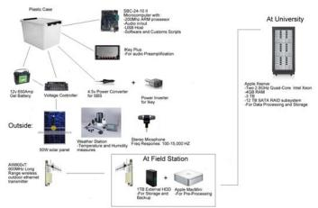
Figure 1. Permanent recording station.
