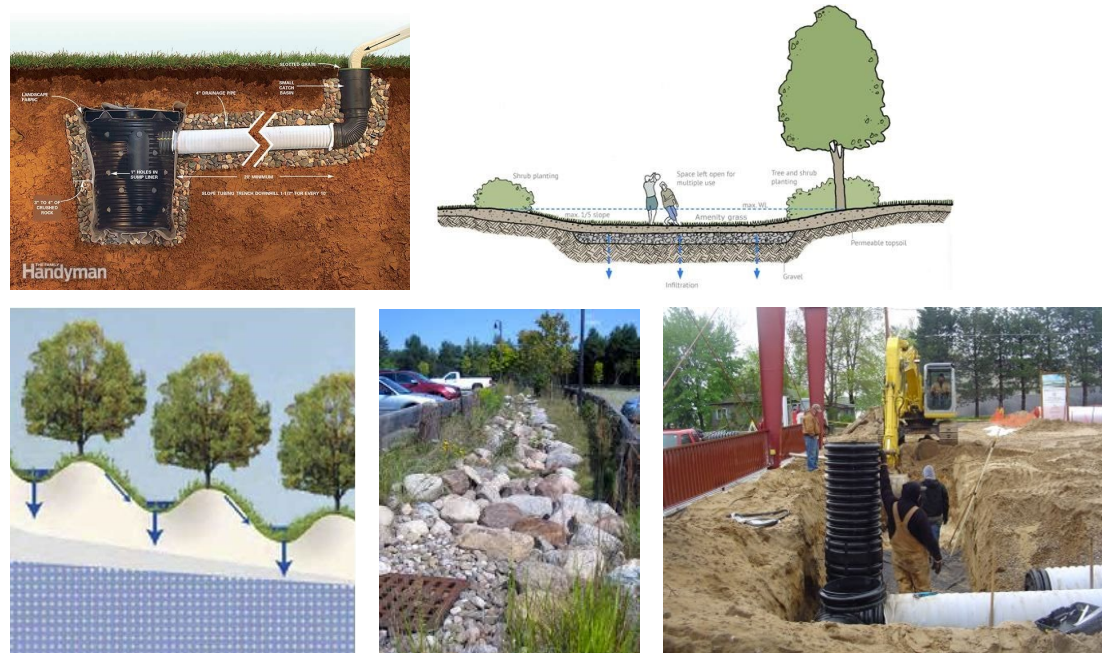
Figure 13. CW from top left, diagram of a dry well, infiltration basin, subsurface infiltration bed, infiltration trench, and infiltration berms.
