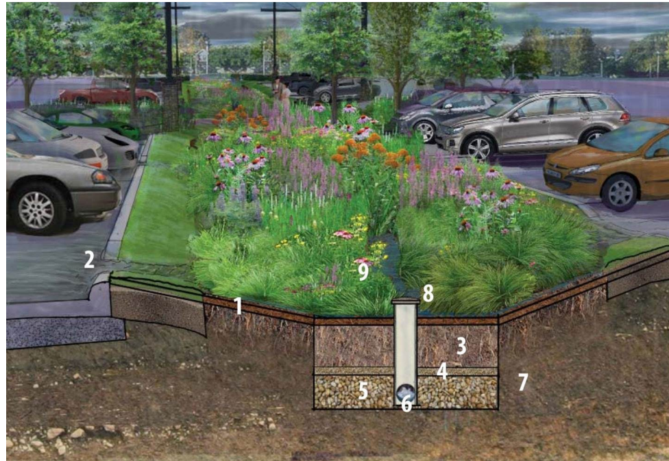
Figure 1. Diagram of bioretention outlining the flow of water through the system (www.jcswcd.org).
