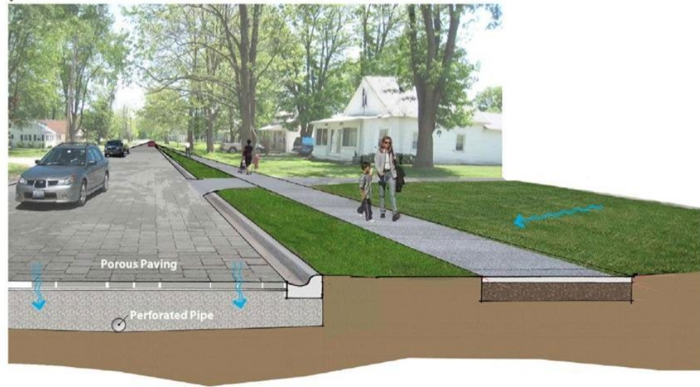
Figure 1. Illustration of how low-volume streets and sidewalks can be retrofitted with permeable pavements ( http://iowaenvironmentalfocus.files.wordpress.com/2011/03/charles-city.jpg ).
