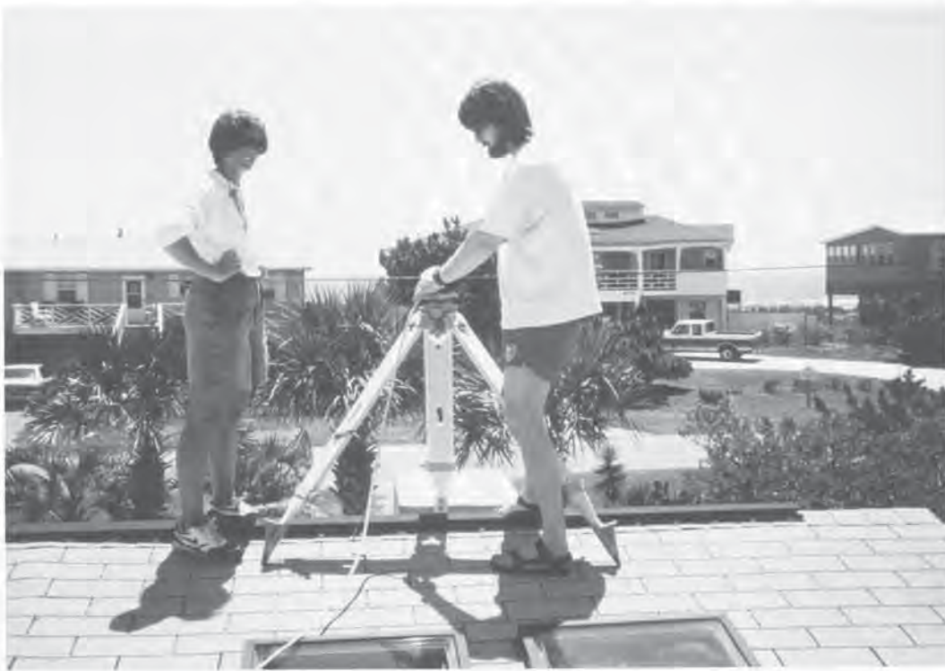
Figure 6.2. Geodesist Tim Smith and a volunteer setting up SCRU's differential GPS base station in Folly Beach. NPS photo by Dave Conlin.
