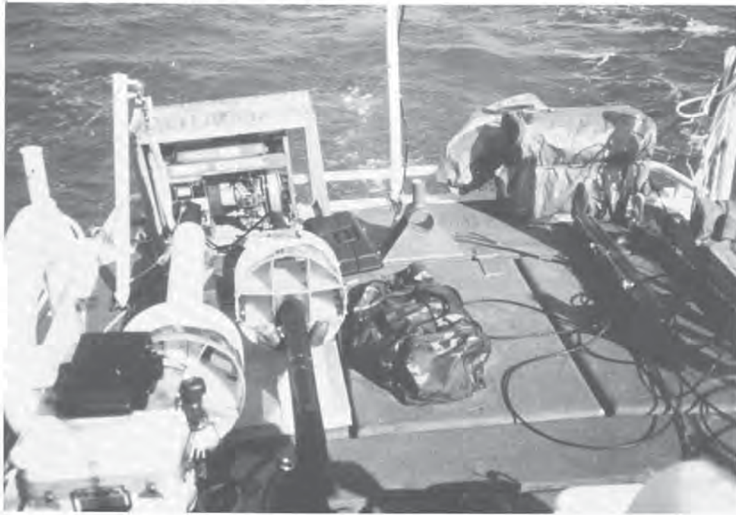
Figure 6.3. SCRU survey equipment on the aft deck of the SCRU survey vessel. Geometrics G-876 magnetometer on left, Marine Sonic Technology side scan sonar on right. Diesel AC generator on left, and a spare under plastic on right. NPS photo by Tim Smith.
