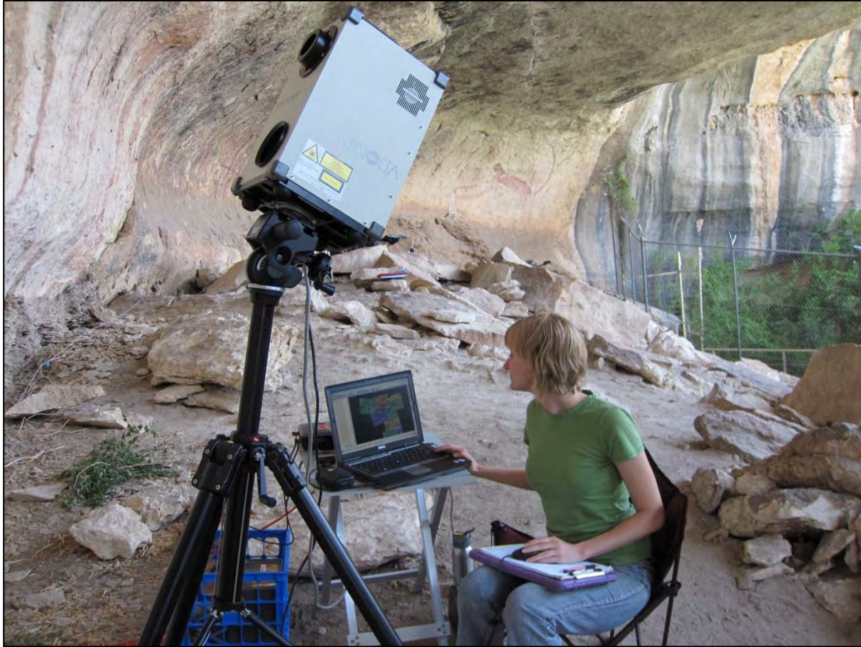
Figure 2.2: Laser recordation performed by Versar, Inc. at Panther Cave, TX.
