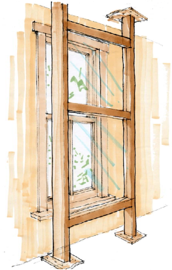
Figure 08 52-4 Possible solution for Force Protection and Anti-Terrorism at an historic building. Build a removable blast guard at the interior of the space, taking care to mimic the configuration of the existing windows.
