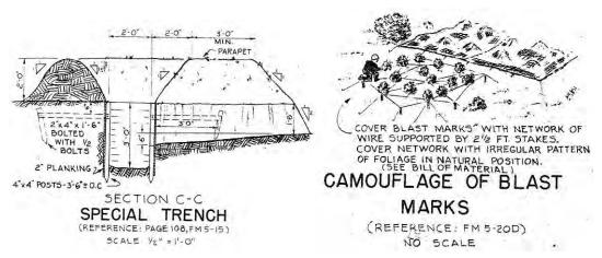
Figure 80. Camouflage demonstration area, 155 mm gun emplacement, special trench and camouflage of blast marks, Fort Bragg, NC, 1952 (Standard Drawing 28-13-80 Sheet 1 of 2, "Details, typical diagram-camouflage demonstration area, 155 mm Gun emplacement," 30 January 1952).
