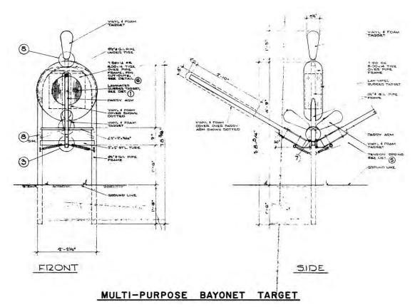
Figure 6. Multi-purpose bayonet target, Fort Bragg, NC, 1966 (Standard Drawing 28-13-117 Sheet 26, "Bayonet dummy—details," 28 June 1966).
