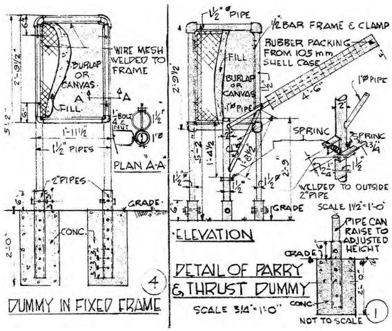
Figure 15. Bayonet assault course, dummy in a fixed frame and details of parry & thrust dummy, Fort Bragg, NC, 1951 (Standard Drawing 28-13-33 Sheet 1 of 1, "Bayonet assault course, typical layout and details," 21 November 1951).
