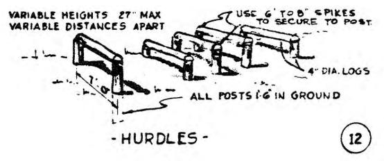
Figure 24. Bayonet assault course, hurdles, Fort Bragg, NC, 1951 (Standard Drawing 28-13-33 Sheet 1 of 1, "Bayonet assault course, typical layout and details," 21 November 1951).
