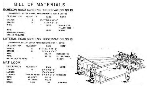
Figure 95. Camouflage demonstration area, bill of materials, echelon road screens, lateral road screens, and mat loom, Fort Bragg, NC, 1951 (Standard Drawing 28-13-67 Sheet 1 of 1, "Details, typical diagram-camouflage demonstration area, road screens and mat loom," 7 December 1951).
