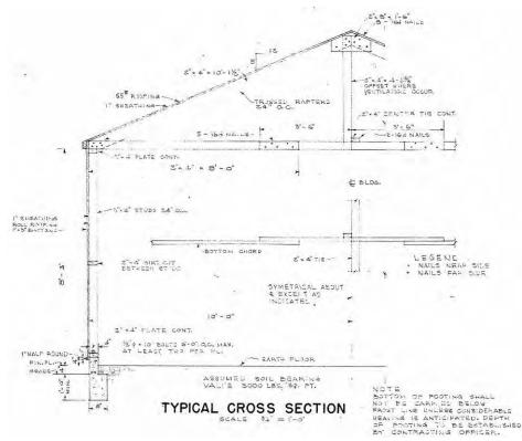
Figure 106. Gas chamber, typical cross section, Fort Bragg, NC, 1952 (Standard Drawing 28-13-46 Sheet 2 of 2, "Gas chamber, details," 28 February 1952).
