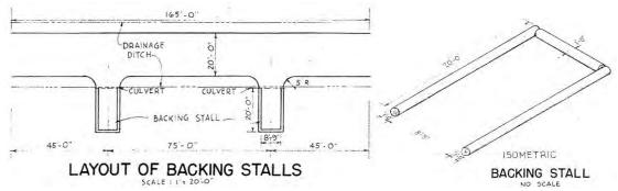
Figure 61. Wheeled vehicle driving course, backing stalls, Fort Bragg, NC, 1951 (Standard Drawing 28-13-50 Sheet 1 of 1, "Wheeled vehicle driving course, plans and details," 21 November 1951).
