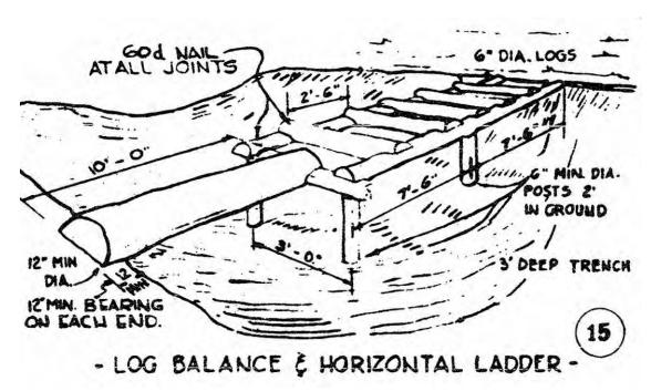
Figure 27. Bayonet assault course, log balance & horizontal ladder, Fort Bragg, NC, 1951 (Standard Drawing 28-13-33 Sheet 1 of 1, "Bayonet assault course, typical layout and details," 21 November 1951).
