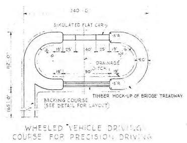
Figure 56. Wheeled vehicle driving course for precision driving, Fort Bragg, NC, 1951 (Standard Drawing 28-13-50 Sheet 1 of 1, "Wheeled vehicle driving course, plans and details," 21 November 1951).
