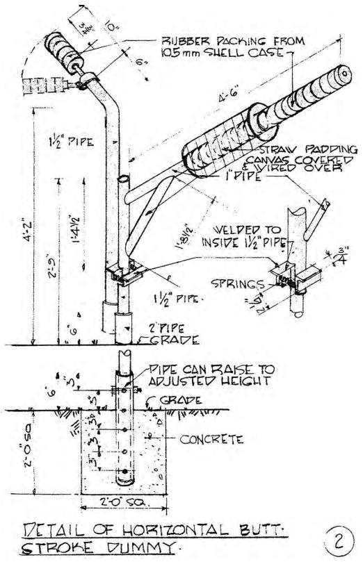
Figure 16. Bayonet assault course, detail of horizontal butt stroke dummy, Fort Bragg, NC, 1951 (Standard Drawing 28-13-33 Sheet 1 of 1, "Bayonet assault course, typical layout and details," 21 November 1951).
