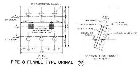
Figure 175. Sanitation display area, pipe and funnel type urinal, Fort Bragg, NC, 1952 (Standard Drawing 28-13-41 Sheet 3 of 3, "Sanitation display area, field facilities, details," 11 April 1952).
