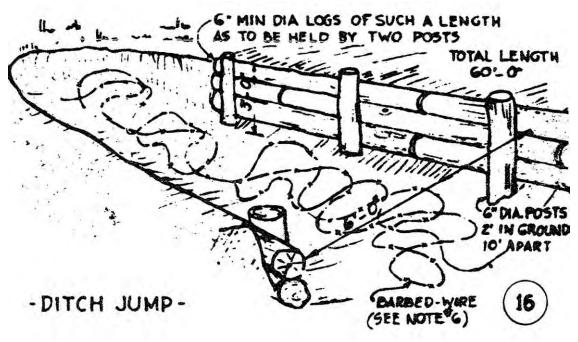
Figure 28. Bayonet assault course, ditch jump, Fort Bragg, NC, 1951 (Standard Drawing 28-13-33 Sheet 1 of 1, "Bayonet assault course, typical layout and details," 21 November 1951).
