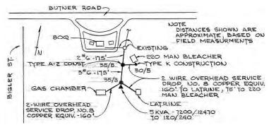
Figure 104. CBR area electrical layout, Fort Bragg, NC, 1966 (Standard Drawing 28-13-117 Sheet 28, "Electrical distribution," 28 June 1966).
