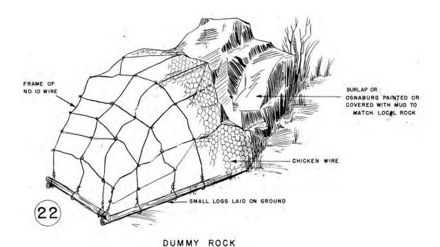
Figure 75. Camouflage demonstration area, dummy rock, Fort Bragg, NC, 1951 (Standard Drawing 28-13-74 Sheet 1 of 1, "Details, typical diagram-camouflage demonstration area, dummy trees, bush, rock and M.G. emplacement," 7 December 1951).
