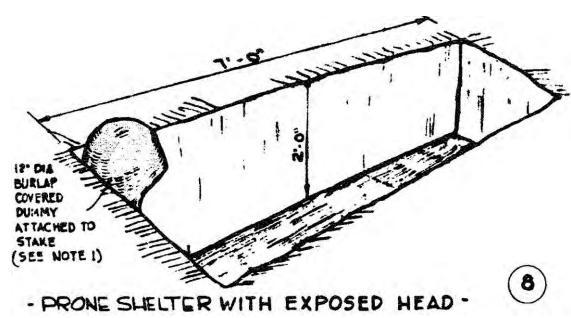
Figure 20. Bayonet assault course, prone shelter with exposed head, Fort Bragg, NC, 1951 (Standard Drawing 28-13-33 Sheet 1 of 1, "Bayonet assault course, typical layout and details," 21 November 1951).
