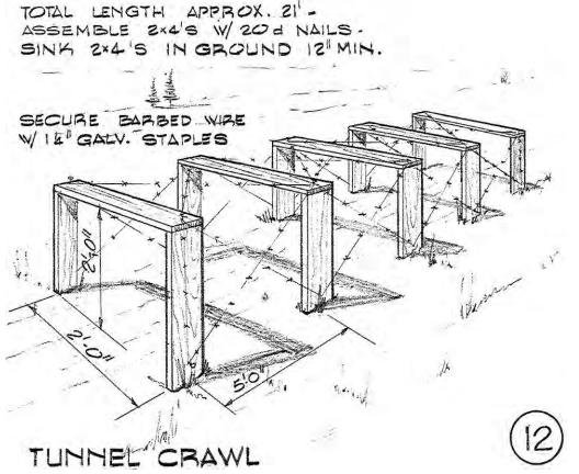
Figure 37. ATC facilities, bayonet assault course, tunnel crawl, plan, Fort Bragg, NC, 1966 (Standard Drawing 28-13-117 Sheet 16, "Construction of ranges, phase 1, U.S. ATC Facilities, Fort Bragg, NC, bayonet assault course," 28 June 1966).
