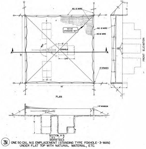
Figure 82. Camouflage demonstration area, one 50 caliber machine gun emplacement (standing type foxhole-3-man) under flat top with natural material, etc., Fort Bragg, NC, 1951 (Standard Drawing 28-13-77 Sheet 1 of 1, "Details, typical diagram-camouflage demonstration area, observation posts and machine gun emplacements," 7 December 1951).
