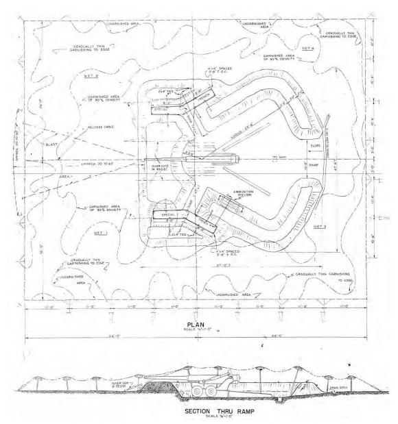
Figure 85. Camouflage demonstration area, 155 mm gun emplacement, plan and section through ramp, Fort Bragg, NC, 1952 (Standard Drawing 28-13-80 Sheet 1 of 2, "Details, typical diagram-camouflage demonstration area, 155 mm gun emplacement," 30 January 1952).
