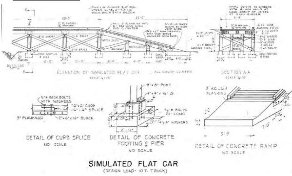
Figure 60. Wheeled vehicle driving course, simulated flat car, Fort Bragg, NC, 1951 (Standard Drawing 28-13-50 Sheet 1 of 1, "Wheeled vehicle driving course, plans and details," 21 November 1951).
