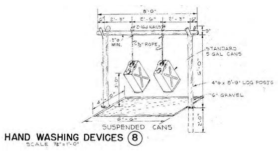
Figure 165. Sanitation display area, hand washing devices, Fort Bragg, NC, 1952 (Standard Drawing 28-13-41 Sheet 2 of 3, "Sanitation display area, field facilities, details," 11 April 1952).
