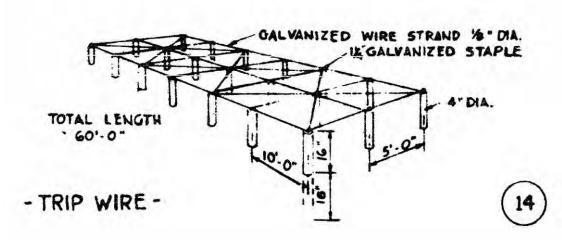
Figure 26. Bayonet assault course, trip wire, 1951 (Standard Drawing 28-13-33 Sheet 1 of 1, "Bayonet assault course, typical layout and details," 21 November 1951).
