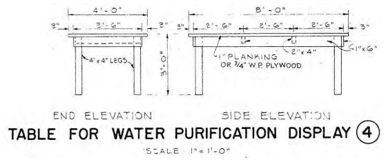
Figure 163. Sanitation display area, table for water purification, Fort Bragg, NC, 1952 (Standard Drawing 28-13-41 Sheet 2 of 3, "Sanitation display area, field facilities, details," 11 April 1952).
