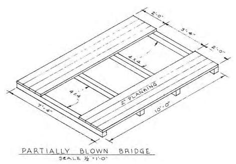
Figure 150. Litter obstacle course, partially blown bridge, Fort Bragg, NC, 1951 (Standard Drawing 28-13-39 Sheet 1 of 1, "Litter obstacle course, layout and details," 21 November 1951).
