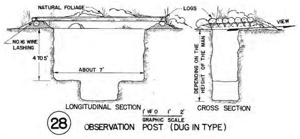
Figure 76. Camouflage demonstration area, observation post (dug in type), Fort Bragg, NC, 1951 (Standard Drawing 28-13-77 Sheet 1 of 1, "Details, typical diagram-camouflage demonstration area, observation posts and machine gun emplacements," 7 December 1951).
