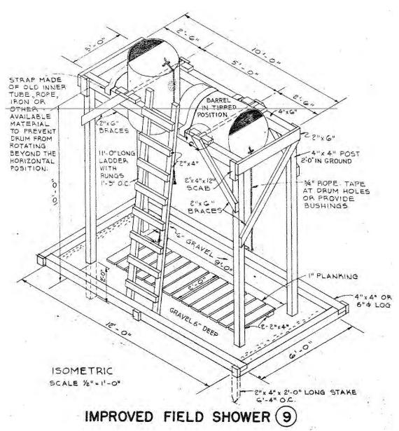
Figure 167. Sanitation display area, improved field shower, Fort Bragg, NC, 1952 (Standard Drawing 28-13-41 Sheet 2 of 3, "Sanitation display area, field facilities, details," 11 April 1952).
