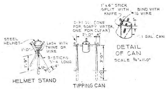
Figure 166. Sanitation display area, hand washing devices, Fort Bragg, NC, 1952 (Standard Drawing 28-13-41 Sheet 2 of 3, "Sanitation display area, field facilities, details," 11 April 1952).
