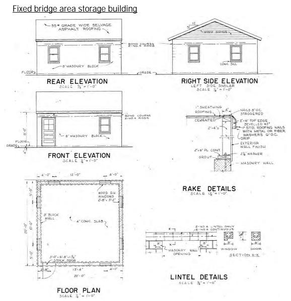
Figure 69. Fixed bridge area, masonry covered storage building, plan, elevations, and details, Fort Bragg, NC, 1952 (Standard Drawing 28-13-97 Sheet 1 of 4, "Bridging area, fixed bridge, covered storage building-masonry," 9 May 1952).
