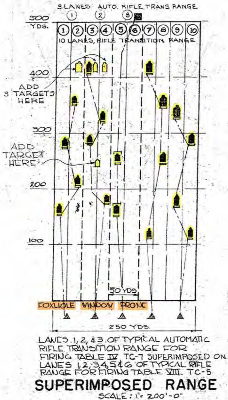
Figure 320. Superimposed transition range, Fort Bragg, NC, 1955 (Standard drawing 28-13-04 sheet 1 of 1, Range, transition, details, 6 June 1955).
