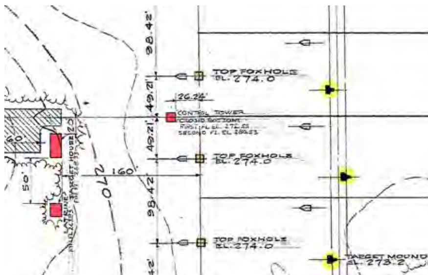
Figure 421. Trainfire ranges record fire No. 1 (12 points), foxholes, Fort Bragg, NC, 1960 (Standard drawing 28-13-115 sheet 2 of 24, Record fire No.1 (12 points), 5 October 1960).
