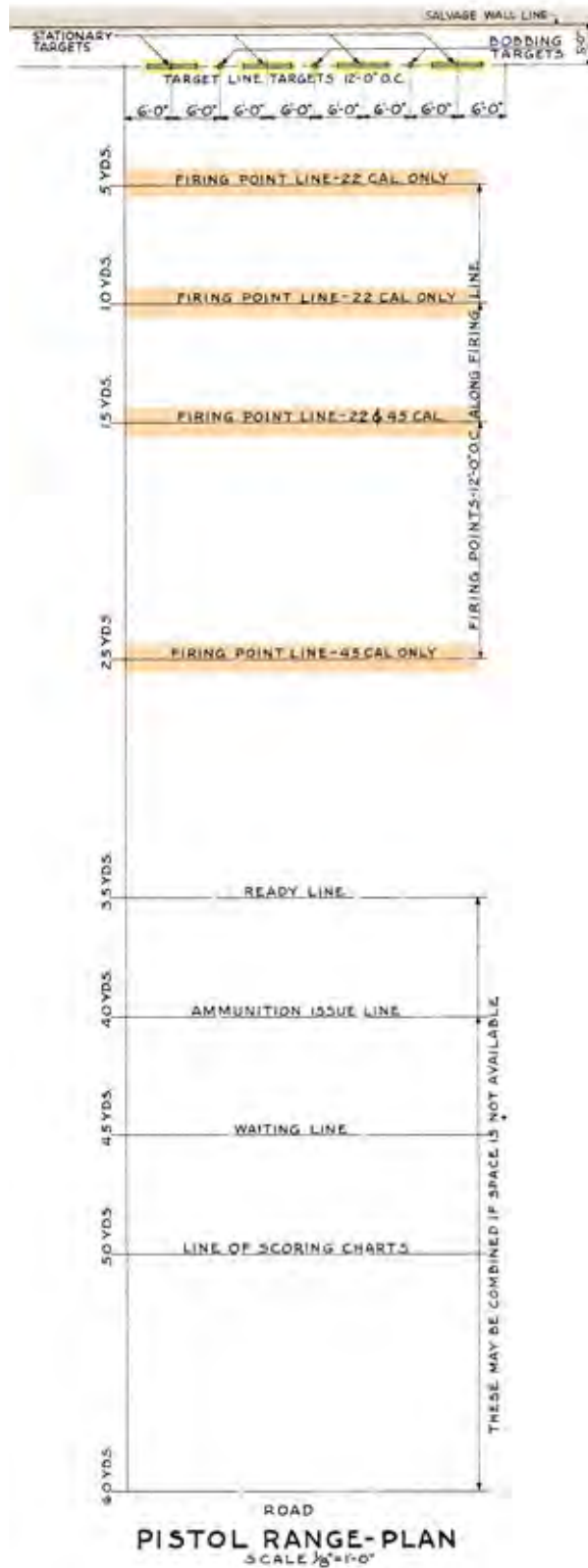
Figure 158. Pistol range plan, Fort Bragg, NC, 1951 (Standard drawing No. 28-13-12 drawing 1 of 1, Range, pistol, landscape targets, plans and details, 21 November 1951).
