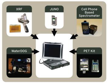
The ETEO will enable rapid environmental data collection from several sensors that can then be automatically aggregated by software for environmental reporting.
