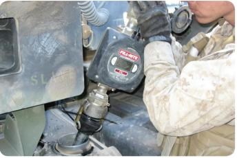
Putting fuel metering system prototype into the hands of an end-user for evaluation under actual operational conditions.
