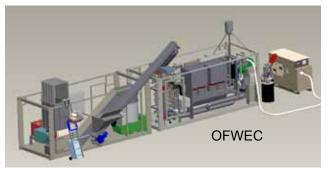
char/ash. The producer gas is very different chemically from natural gas, but both can be burned to provide heat and/or power. The OFWEC gas is sent to a standard Army-issued 60-kilowatt Tactical Quiet Generator (TQG) adapted for bi-fuel operation.
