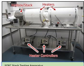
**SOFC Stack Testing Apparatus**
