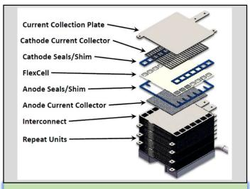
**Expanded View of SOFC Stack**
