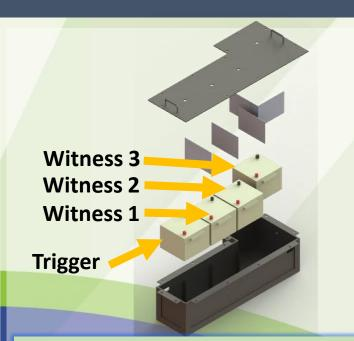
Exploded view of Stryker vehicle test fixture with four Toshiba Li6Ts batteries
