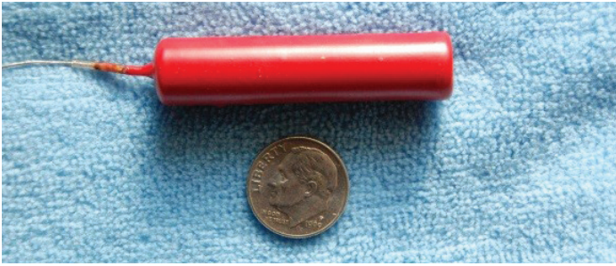
Example of radio transmitter used to monitor the snakes. Photo by: Chris Petersen, DoD PARC
