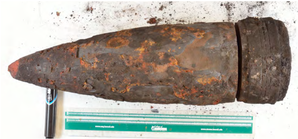
Figure 1.2. Munition casing evaluated during this effort. This 5” AP shell was further subsampled and cross-sectioned for corrosion analyses.
