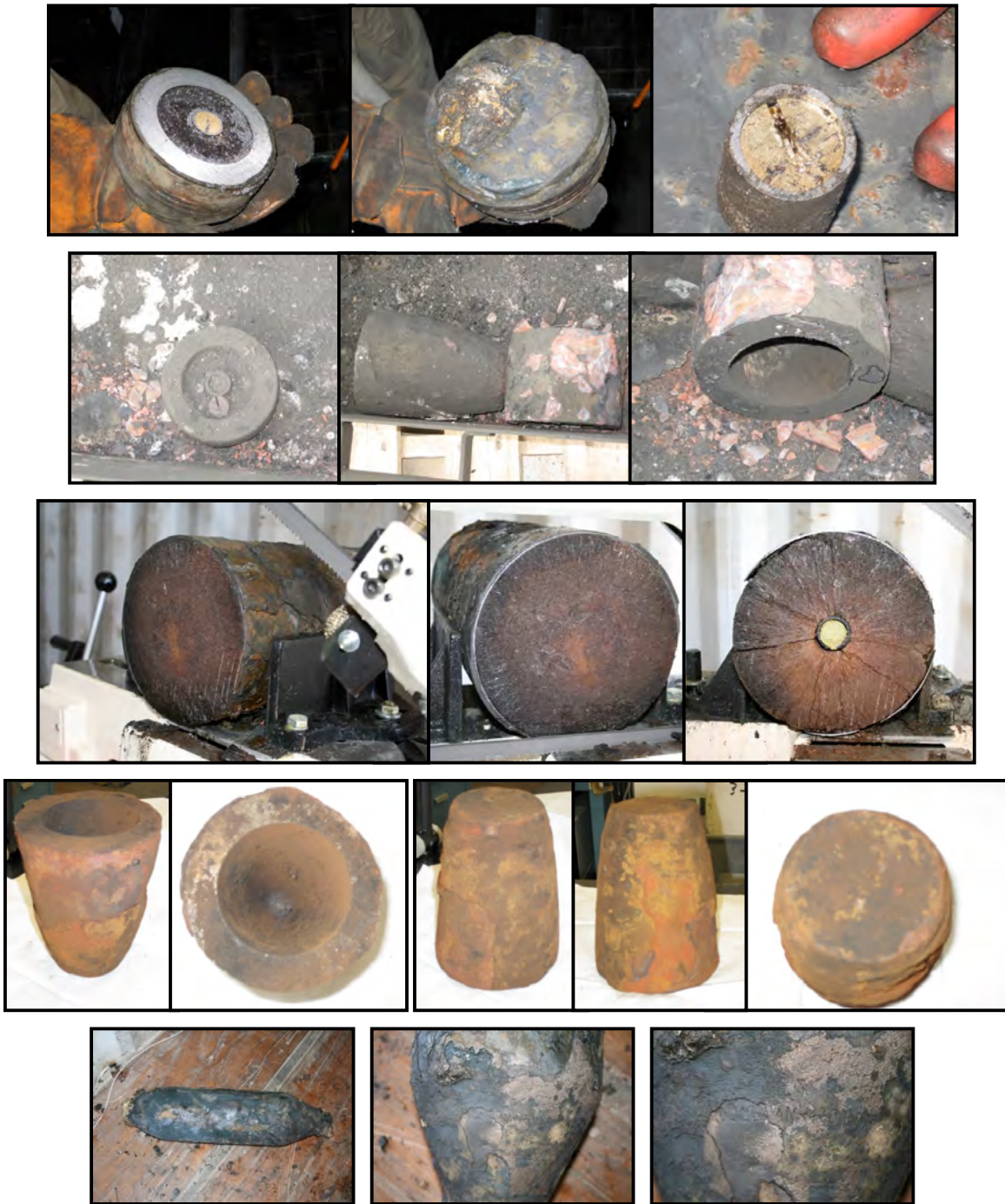
Figure 2. Examples of field-collected EHDS-treated munitions casings for corrosion studies. Samples collected and treated at the site were subsequently photo-documented and down-selected for corrosion studies at the Hawai'i Corrosion Laboratory (HCL).
