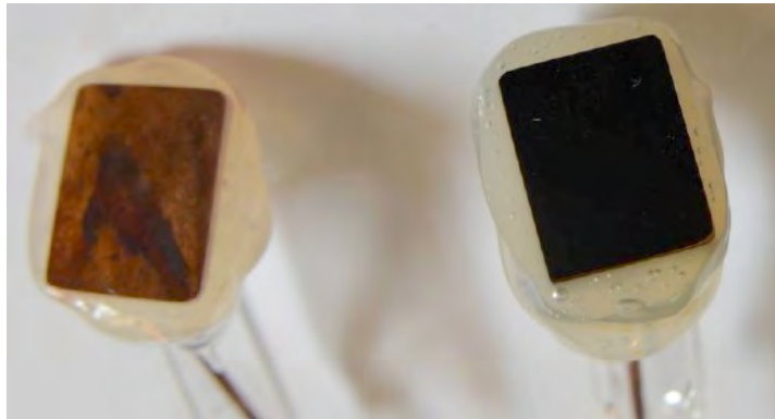
Figure 3.3. A typical steel and copper electrode
