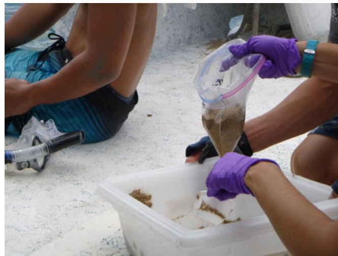
Photo 4: Transferring sediment collected by the PONAR into a sealed bag.
