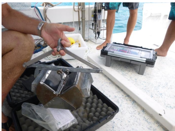
Photo 3: PONAR used for sediment collection at the NPS stratum.
