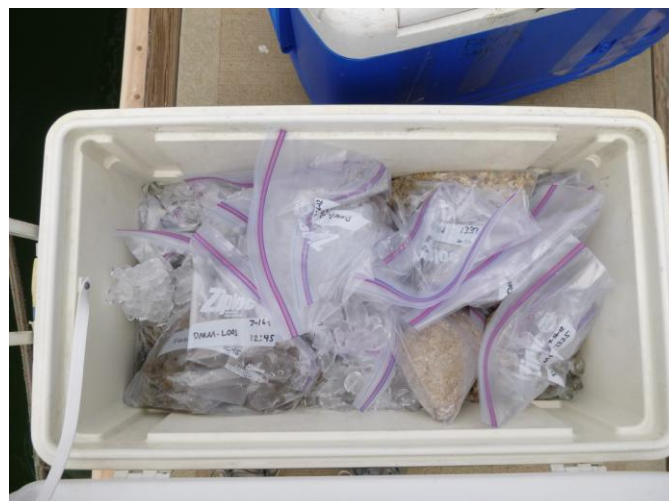
Photo 6: Sediment and biota samples double-bagged and preserved on ice in the cooler.
