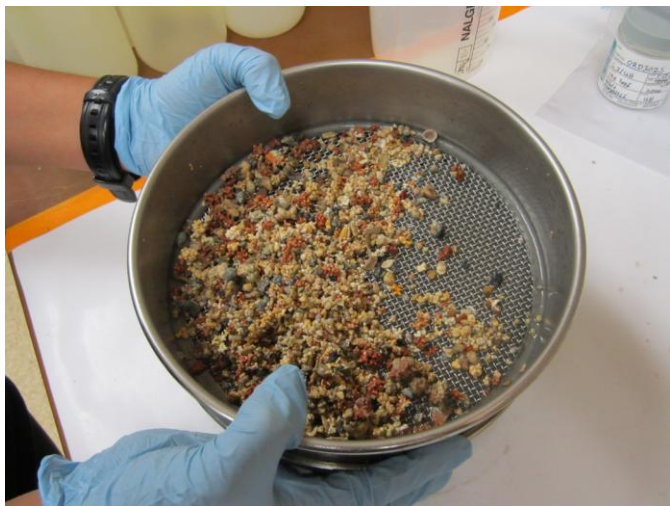
Photo 14: Sieving sediment samples through a 2 millimeter screen sieve.
